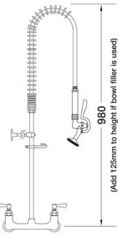
2x (F) 1/2-inch connections Tap hole req.: 2x 25mm dia.
