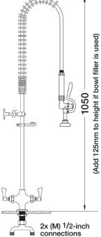
**Tap hole req.: 30mm dia.**Dimensions are in millimeters. If a Cad file is required please visit <u>www.mechline.com</u>.
