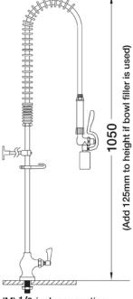
(M) 1/2-inch connection Tap hole req.: 25mm dia.
