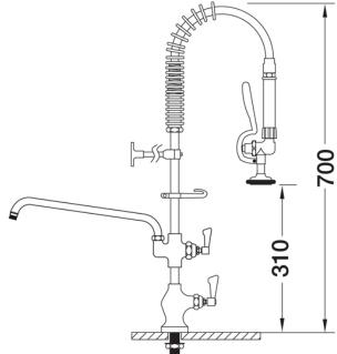
(M) 1/2-inch connection Tap hole req.: 25mm dia.
