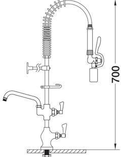
(M) 1/2-inch connection Tap hole req.: 25mm dia.
